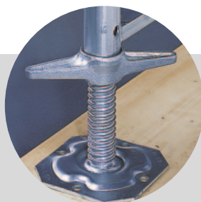
Self cleaning adjustable base plates (rolled thread) with ident mark preventing over-extension.
