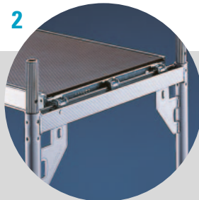
The 3 claws of the deck (0.61 m wide) slip easily and safely into the U-profile of the frame.
