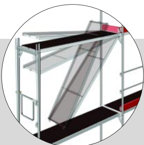
Individual bays can be attached or removed without dismantling the entire scaffold.
